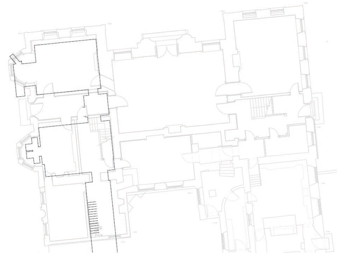
Plan. 5.5. Cellar plan. The two large cellar chambers fill the western section of the 'H' plan; the contemporary cellar passage to the south is now beneath an additional room of 1754.
